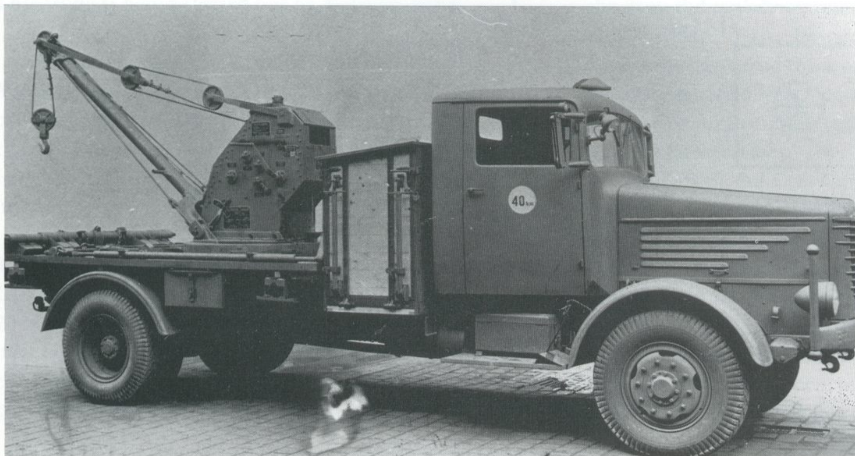
Rotary crane truck with a lifting capacity of 3 tons, based on a Büssing-NAG 4.5 ton chassis, Type 4500 A.
