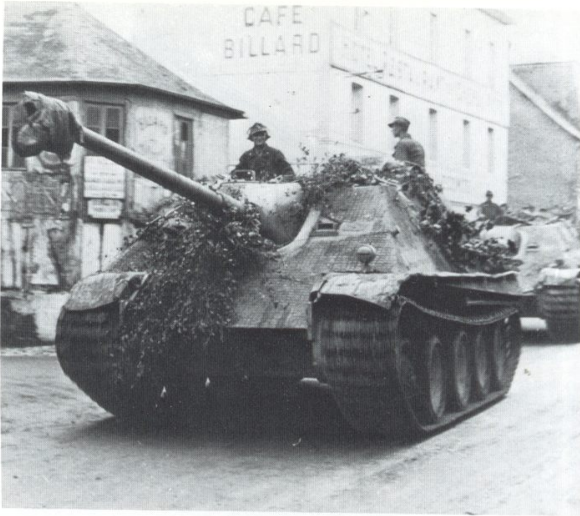
Jagdpanthers during operations in Normandy. Notice the covered outer driver's vision block.
