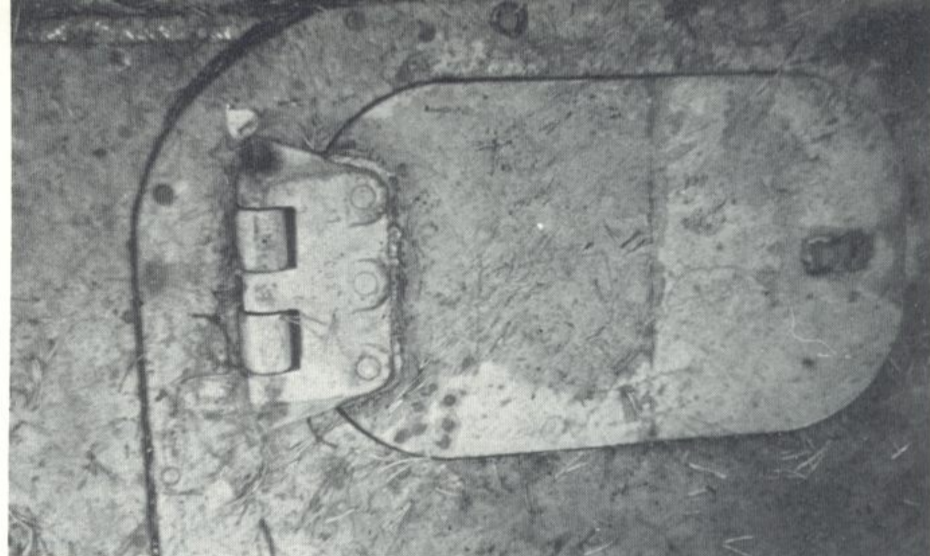
Driver's and radio operator's entry hatches, modified beginning on the G model. Here in closed position (radio operator's on the left, driver's on the right)
