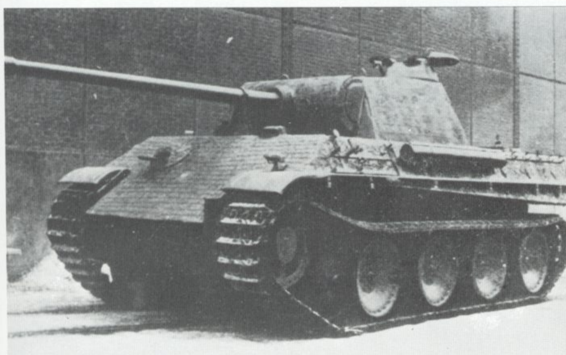
This side view of a G model shows the downward angled edge of the tank hull above the running gear.
