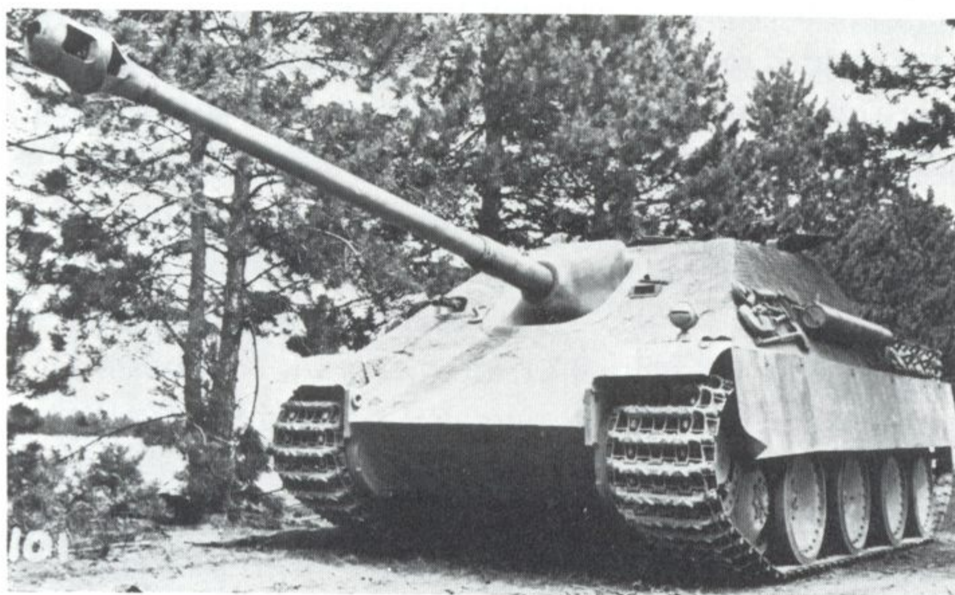
Later models had only one opening for the driver's optics and two-piece barrels for the 88mm Pak.
