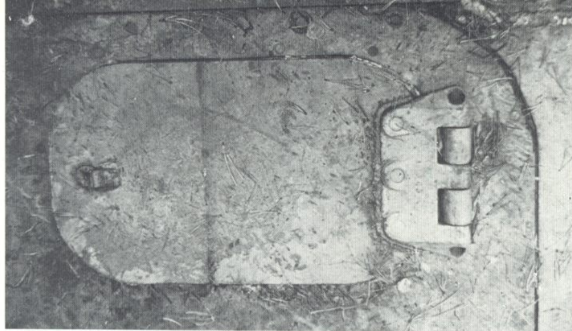
Driver's and radio operator's entry hatches, modified beginning on the G model. Here in closed position (radio operator's on the left, driver's on the right)
