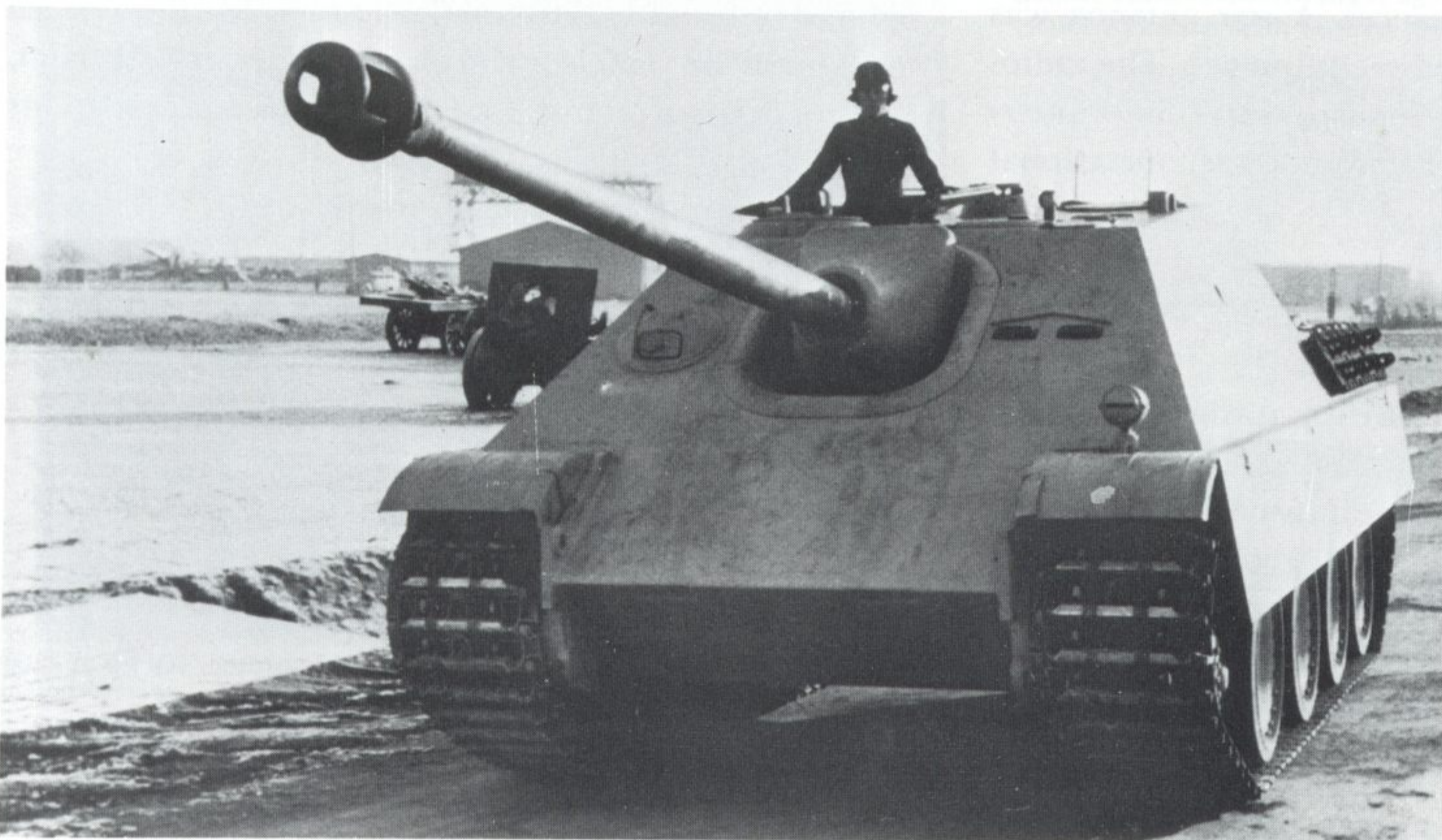
One of the initial Jagdpanther vehicles as evidenced by the double driver vision ports and the pistol port on the side of the superstructure.
