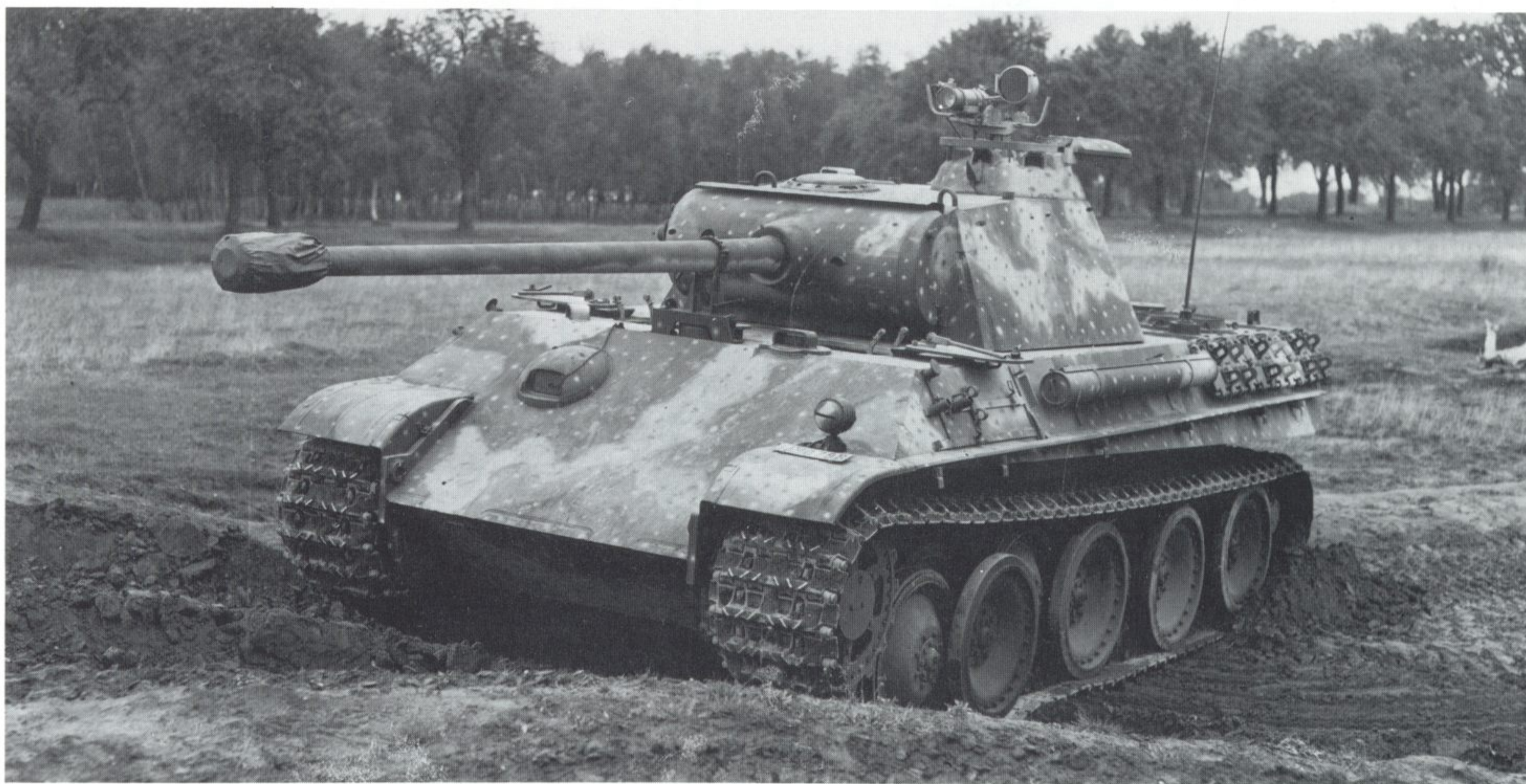
Panzerkampfwagen Panther Ausf. G with infra-red gunsight and headlamp mounted on the commander's cupola.
