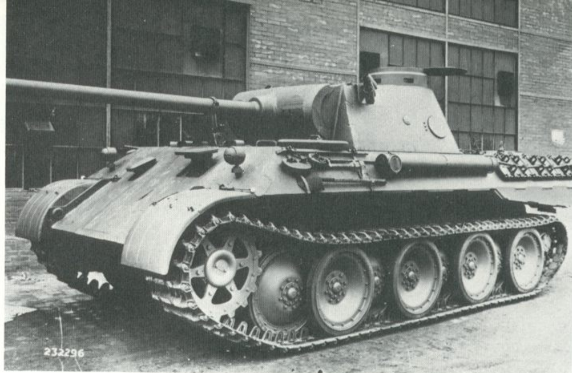
One of the first Panthers built by MAN shows the layout of tools and other equipment on both sides of the vehicle.
