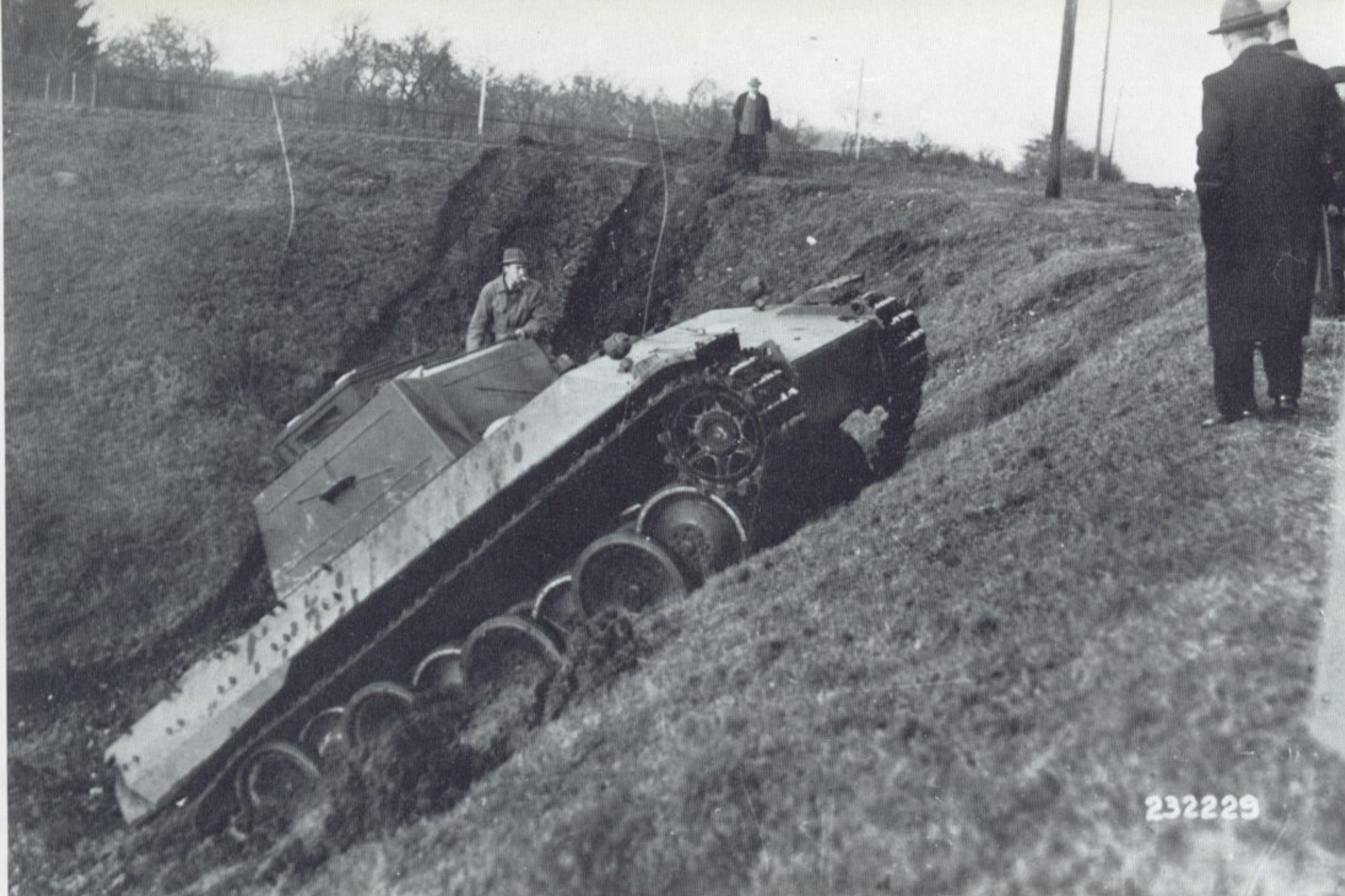
First MAN VK 3002 prototype during factory trials.
