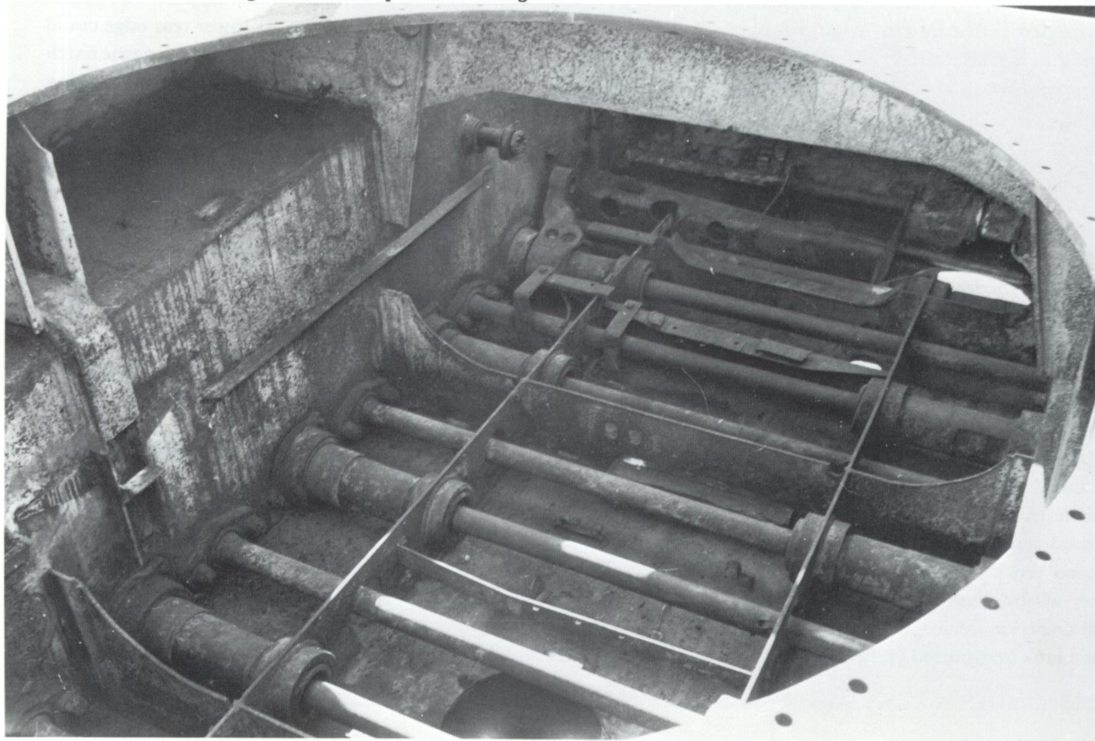
The Panther II had the single torsion bar suspension of the Tiger B.
