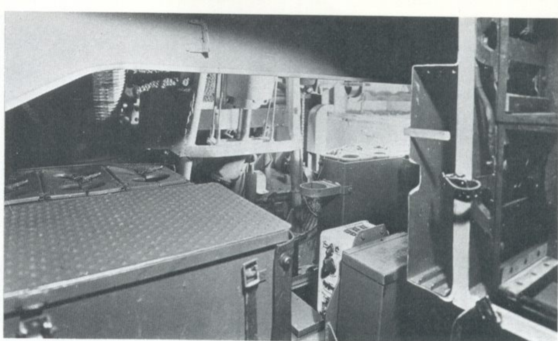
Details of the fighting compartment showing ammunition racks and other equipment items.
