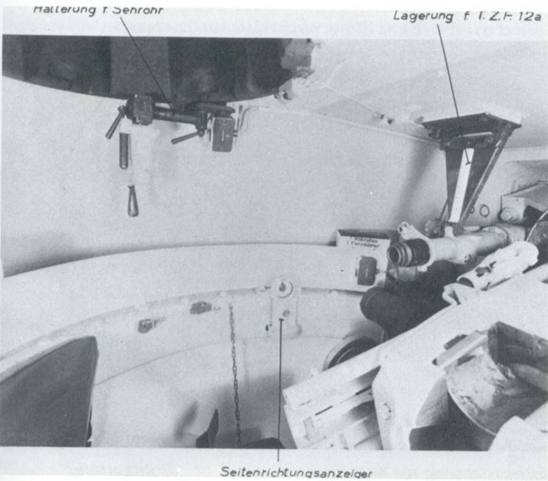
Mounting for the turret gunsight. The azimuth indicator has only one gauge in this version.
