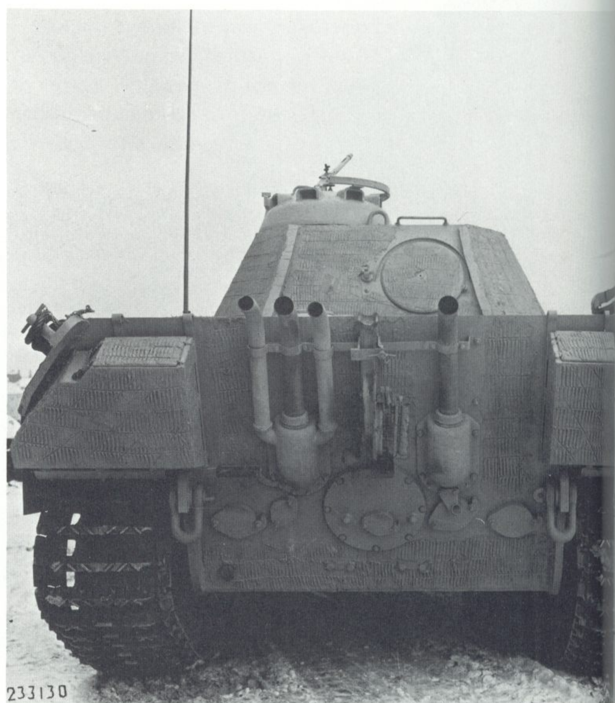
These rear end photos of a Panzerkampfwagen Panther Ausf. A show the improved exhaust cooling in the right photograph and the different method of carrying the jack so as to improve accessibility to the maintenance openings.
