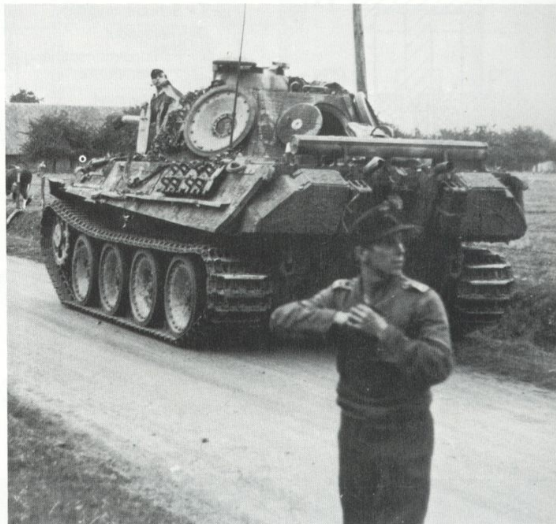
Some G models had the container for the gun cleaning equipment mounted crosswise over the engine compartment.
